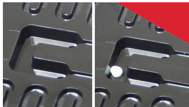
Cartridge chamber with and without pellet.
