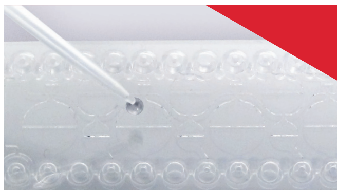
Reagent being pipetted into a cartridge.
