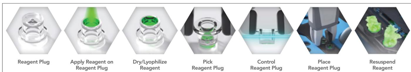
Figure 4 — Dry Reagent Preparation and Resuspension
